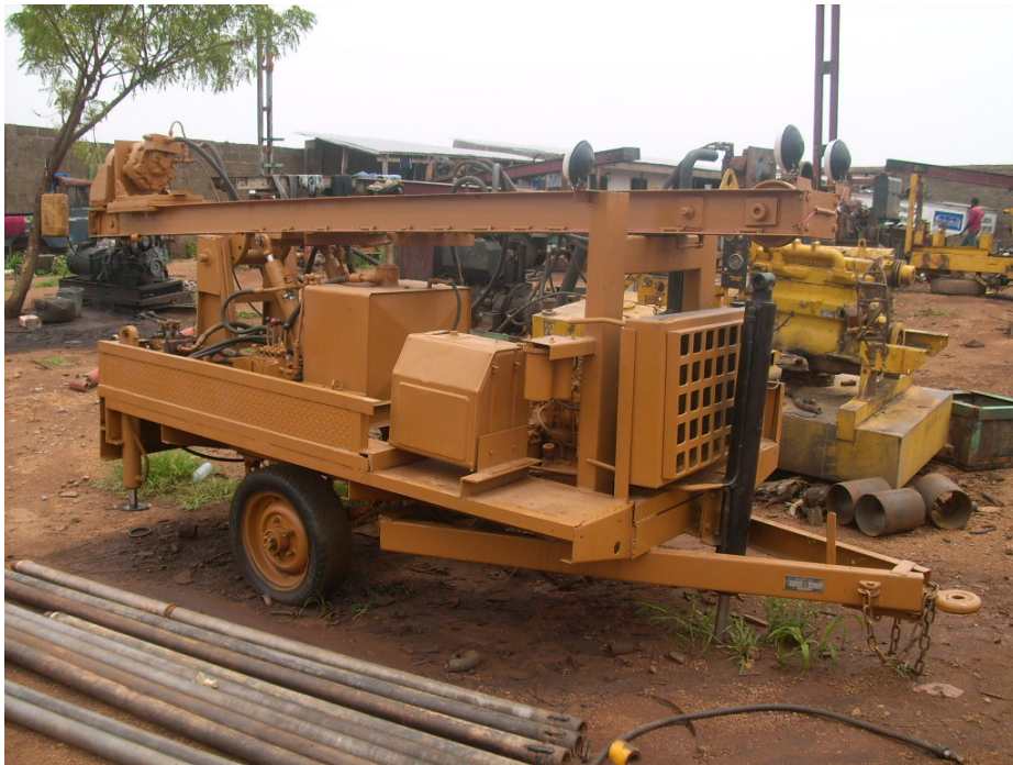
Picture 1 Trailer rig from A.U Drilling in Kaduna
